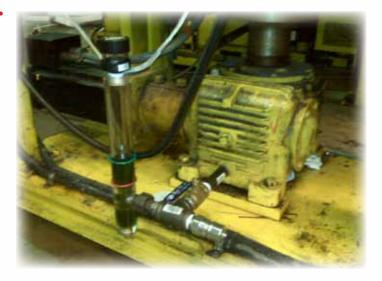
Mark recommended that all the gearboxes be flushed with LE's Monolec<sup>®</sup> R&O Compressor / Turbine Oil (6405) at no load, and then drained. After the flushing, he recommended the use of LE's Monolec Synthetic Industrial Lubricant (9460) in the cone drive.
